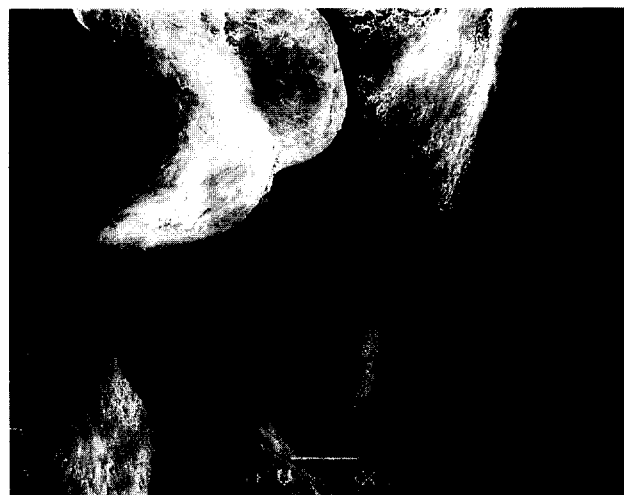
Figure 7 SEM photograph of an UHMWPE UH210 sample compacted at 90.9 MPa and 127°C for 30 min. The magnification of the photograph is 1200
